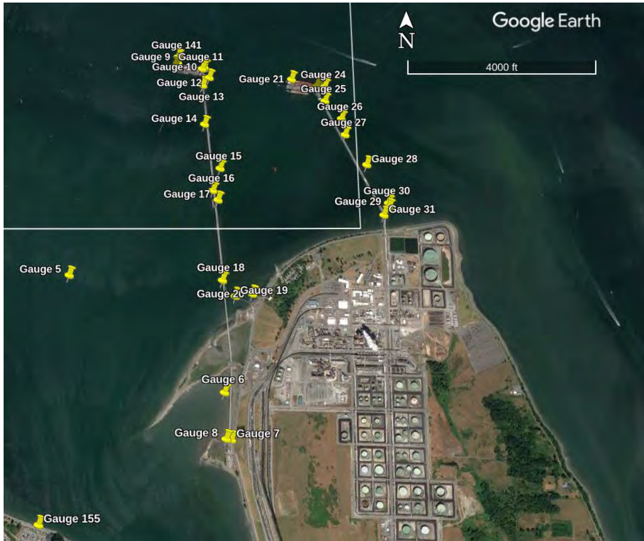
Figure 16. Gauges around March Point. Gauges within the white rectangle in the northwest corner of the map are modeled at 1/9 arc-second resolution. Other gauges outside of white rectangle are modeled at 1/3 arc-second resolution.
