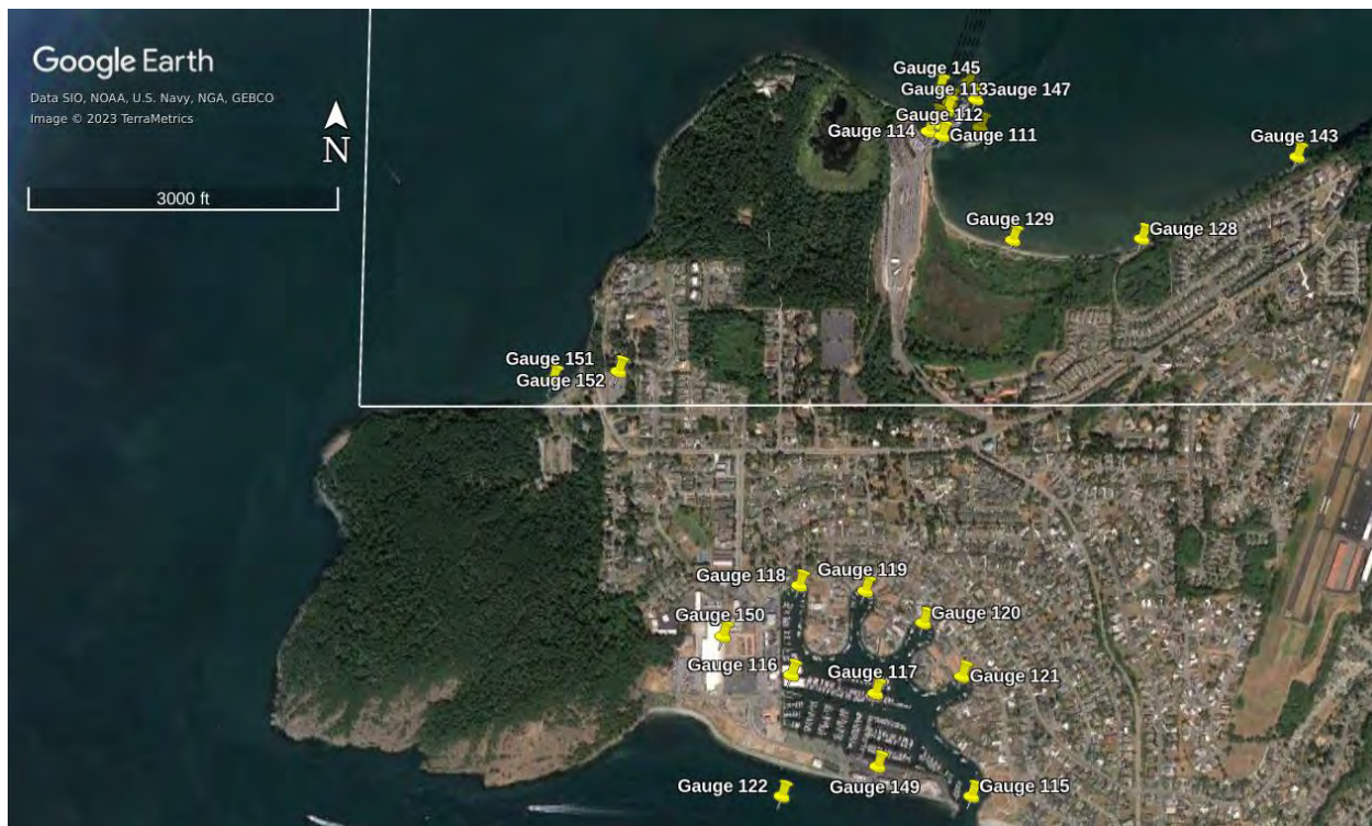
Figure 17. Gauges around Fidalgo Head. Gauges within the white rectangle in the northeast corner of the map are modeled at 1/9 arc-second resolution. Other gauges outside of white rectangle are modeled at 1/3 arc-second resolution.
