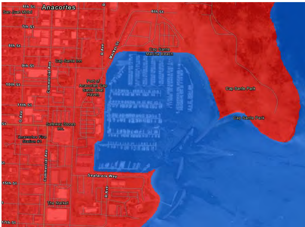
Figure A1. Top: Aerial imagery of Cap Sante Marina at the Port of Guemes Channel. Bottom: Original unmodified DEM extent covering Cap Sante Marina. Red areas are elevations greater than MHW and blue areas are elevations less than MHW.
